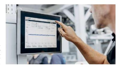
The inline viscometer "Visco P" measures the actual viscosity under processing conditions and in real time (All images: Promix Solutions AG)
