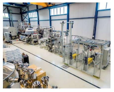
of post-consumer PET flakes for food packaging, combining crystal-lization and drying in a single process. The system operates without vacuum technology and can be retrofitted on existing extrusion lines. The efficiency of the cleaning process has been verified by a Letter of Non-Objection from the US Food and Drug Administration (FDA), while tests have shown compliance with the European Food Safety Authority (EFSA) criteria for the use of recycled materials for direct food contact packaging.
