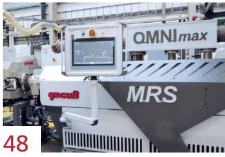
Gneuss' MRS Extrusion Technology is known as an alternative for the reprocessing of contaminated materials. In combination with Gneuss' Rotary Filtration Systems, vacuum technology, an online viscometer and Measurement Technology, customizable recycling lines tailor-made for a specific material can be engineered
