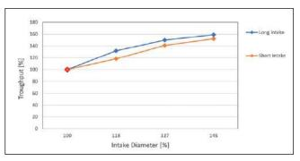
Diagram 2: Influence of the EVI diameter and length on the machine throughput
