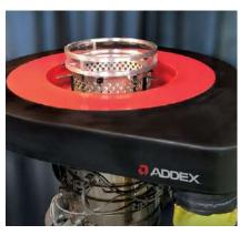
multi-inlet plenum. The company's new aerodynamic design (patent pending) employs dual counterflow channels which direct air flow in two opposing directions inside the plenum. These two counterflows of air join inwardly together to create a combined uniform flow of air to the lip set. The measured overall profile performance is better than with a conventional multi-inlet air ring and inlet effects aren't seen in the film which is a major step forward in single-inlet plenum design.
