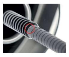
Also extremely small flaws, like the above shown tiny dent in protective tubing for electronic wiring in cars, may easily become safety-critical. ProfilControl 7 S CorrugatedTube assures the quality of corrugated tubing for use in automotive engineering and other demanding applications
